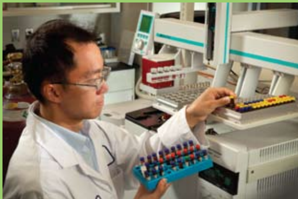
Quality Control Technician Raymond Lee loads samples into the gas chromatography mass spectrometer. Examining chemical profiles is part of the ChemBioPrint process of chemical and biological standardization.
